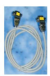
Half duplex communication, with RTS/CTS Handshake is implemented. The RS232 port has a DB-9 female connector and standard communication is implemented as (115200 N 8 1):
